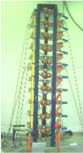
Impulse voltage generator.
